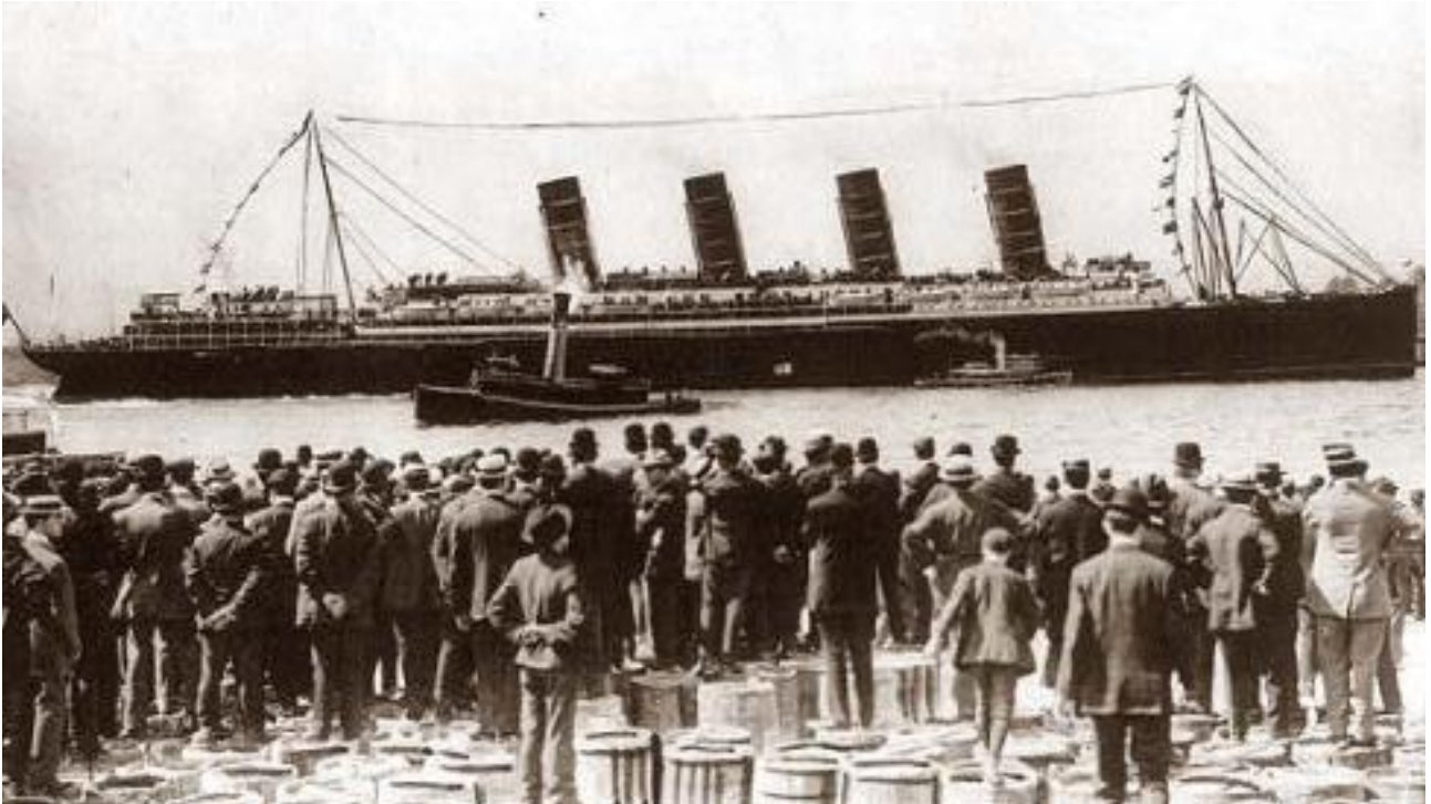
The Lusitania had four screws, with one boiler room and one funnel for each—unlike the Titanic which had only three screws but was given a fake fourth funnel
