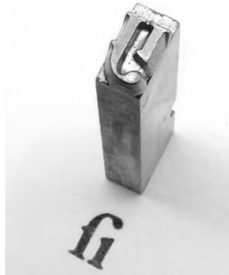
(Above) The letters “f” and “i” do not sit well together, so here is the solution, the “fi” ligature as it might appear in print; on the right is the single block of lead type for this ligature; (below) some ligatures are more commonly used than others
