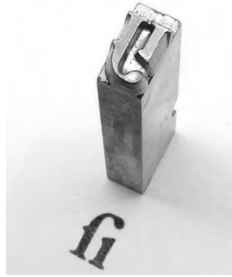
(Above) The letters “f” and “i” do not sit well together, so here is the solution, the “fi” ligature as it might appear in print; on the right is the single block of lead type for this ligature; (below) some ligatures are more commonly used than others
