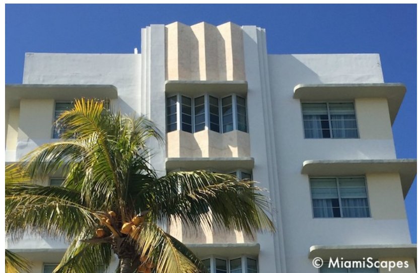
(Above and below) famously inexpensive Art Deco buildings in South Beach, Miami, showing characteristic easily-constructed, low-maintenance “eyebrows”
