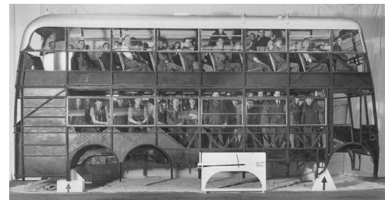
Leyland has shepherded 77 members of its factory staff into the almost complete body of an unidentified F1. The occasion was a stress test on the steel framework which was supported at just two points (marked by arrows), one under each main bulkhead
