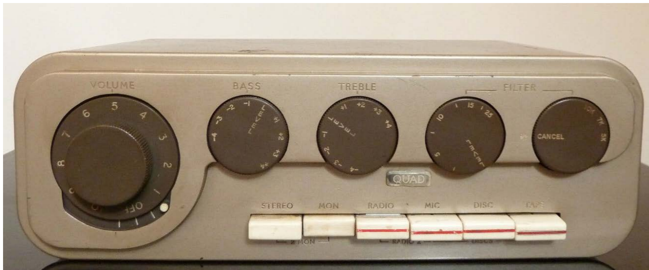
(Above) The Quad 22 preamplifier, introduced in 1958 to cope with stereo sound sources
